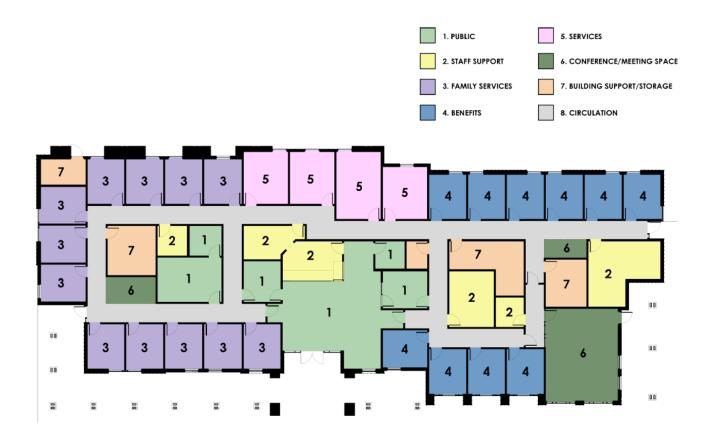
Ms. Adams showed the training/conference space at the bottom right of the diagram as the green space with the number 6. She explained that the training space was placed the on an exterior wall to provide the option for potential use for afterhours.
